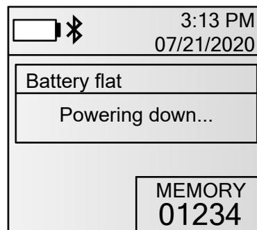
*Note: If the battery level is critically low (0%), the reader will not power up.*
