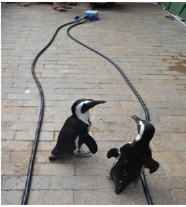
The Biomark **Cord Antenna System** is a portable PIT tag detection system with a flexible cord antenna designed for a variety of monitoring applications. It is quick and easy to deploy, and commonly used to detect PIT Tagged fish and wildlife in streams, caves, wildlife crossings, and other unique places.
