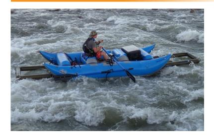
Biomark **Rigid and Inflatable Floating Antennas,** are an innovative approach to both stationary and mobile PIT-tag monitoring. The rigid design is made up of a 10' HDPE antenna affixed to an FRP framework and is ideal for semi-permanent, multi-antenna arrays and larger river/higher flow applications.
