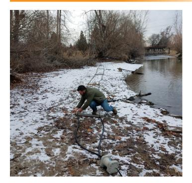
The Biomark **LITZ CORD** corded antenna can be configured with the IS1001 reader housed in a shorebased enclosure or with the IS1001 in a submersible enclosure. Due to the interaction between antennas when in a pass-by orientation, the antenna can only be deployed as single standalone units and not multiplexed or synchronized with other pass-by antennas.
