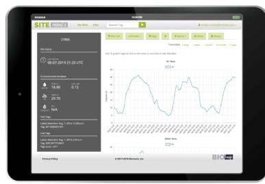
Biomark's **BioLogic Site Module** provides near real-time access to view status of remote PIT-tag detection sites. Data is retrieved every 4-hrs and displayed in the web portal. BioLogic Site Module is an effective tool for managing O&M labor and minimizing downtime; resulting in a robust dataset.
