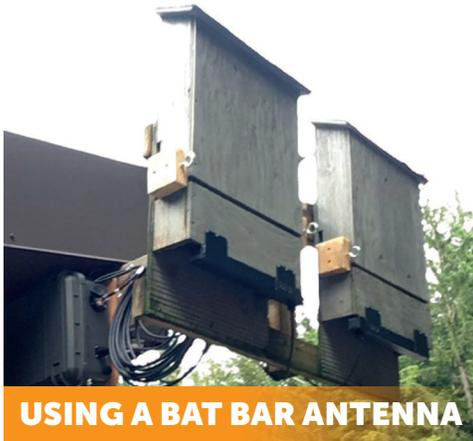
**USING A BAT BAR ANTENNA**
